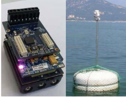
Figure 4: IMote2 sensor and a deployed sensor buoy
